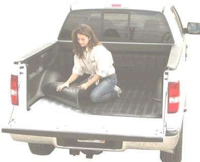
The next step is installing the tailgate panel. **If your truck is equipped with a tailgate step, you will not use the tailgate panel.**
