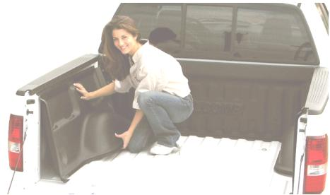
Align the holes in the sidewalls with the holes in the loadguard. You may use a Phillips screwdriver or punch as an alignment tool.
